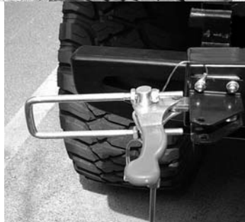
Latch and latch-plate >>> Adjust latching "U-bolt" so it takes no more than 25lbs to latch handle and remain closed. More than this amount of torque to latch could result in damage to the "U-bolt" and / or latch-plate and bolts over time.
