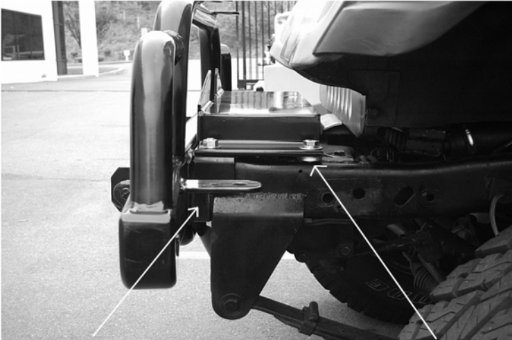
Note custom spring hangers and necessary notching in bumper mounting brackets. Although this is an extreme case, there are instances where stock hangers/shackles contact the bumper mounting brackets.
