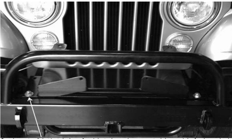
Front bumper installed with winch-plate - front holes in plate use bumper mounting bolts, rear holes for plate need to be drilled. Brackets will be available in the future to bolt into the side of the frame-rail - contact us for availability.
