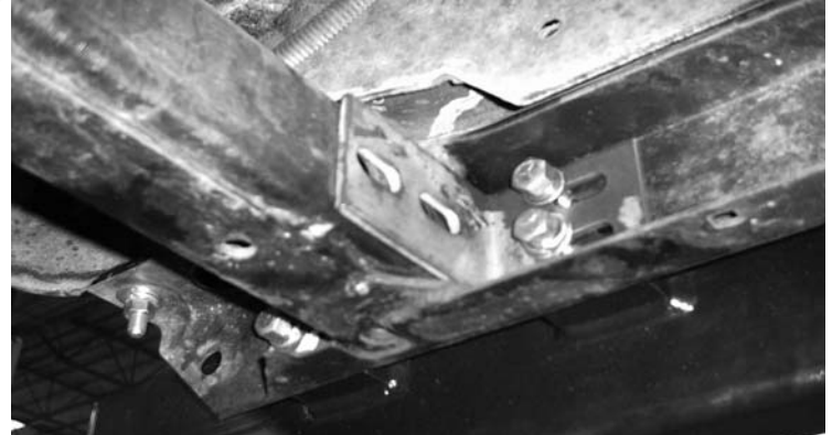
Passenger side frame-rail - CJ8 shown with alternate bolt-pattern. Frame support-brackets shown unpainted for photo purposes.
