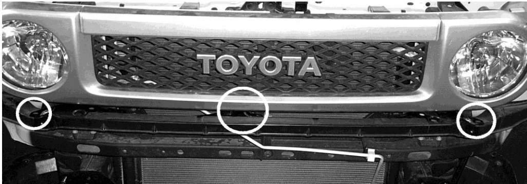
Photo 2 - Unclip bumper fascia from fascia support bracket through removed grill opening.
