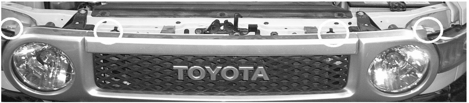
Photo 1 - Remove the "push-pins" from grill mounts outside of headlights. Remove the hold-down screws at the top inner edge of grill (all circled in white above). Remove the grill by popping the snap-clips (2 on each side just inside the headlights) and pull forward off your FJ.
