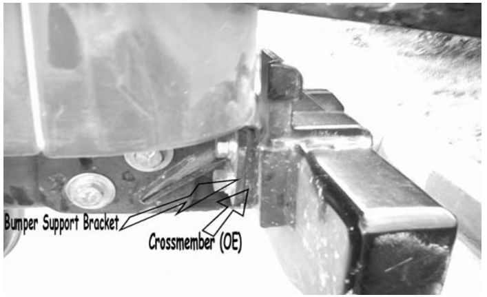
05-06 TJ owners with canted crossmember - install spacers or washers between crossmember and bumper on upper bolts only.
