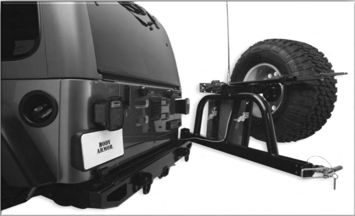
Bumper and optional Tire/can Carrier PN 5292 shown on installed on TJ
