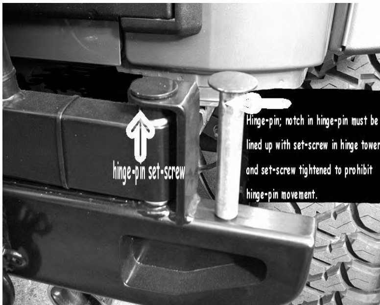
Photo 1 - Hinge-pin and tower set-screw. It is critical that hinge-pin be installed so the notch lines up with the set-screw in the hinge-pin tower, and the set-screw is tightened into this notch. Photo
