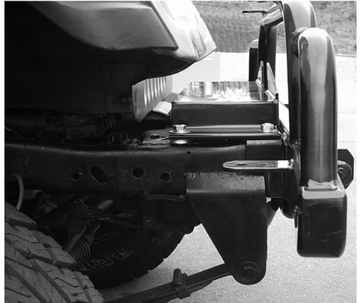
Above photo reflects winch plate mounting - Passenger side CJ*
