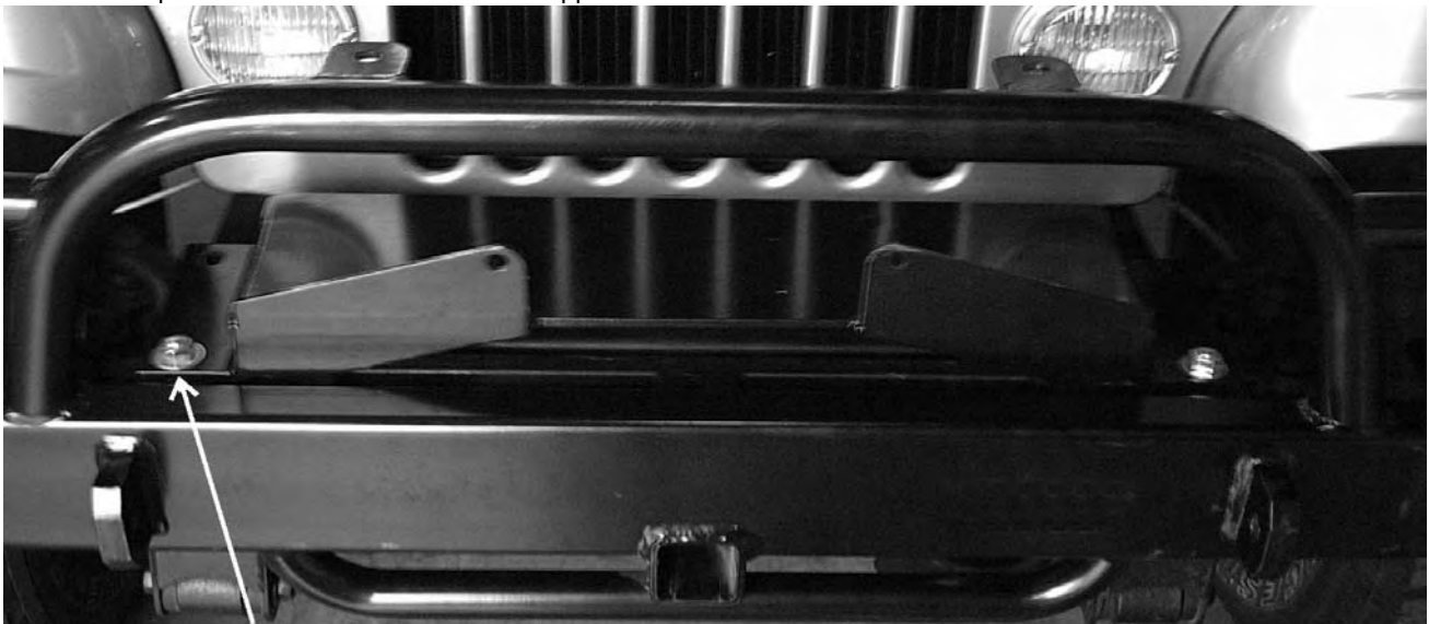
Above photo reflects winch plate mounting - Driver side CJ* The rear holes for the plate on this CJ were drilled and tapped for aesthetic reasons.
