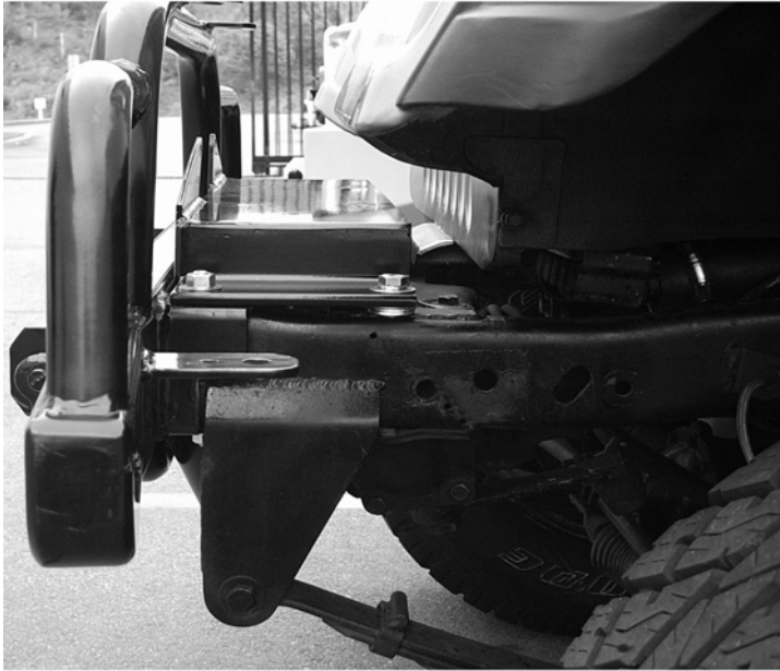
Above photo reflects winch plate mounting - Driver side CJ* The rear holes for the plate on this CJ were drilled and tapped for aesthetic reasons.
