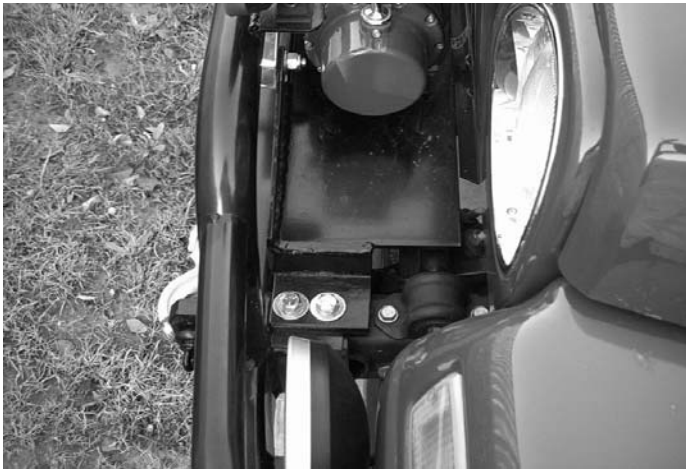
Above photo reflects winch plate mounting - Driver side TJ*
