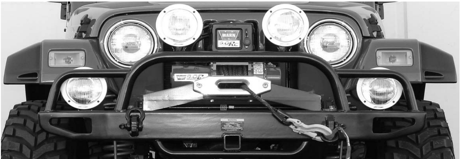
Above photo reflects front installation detail with Warn's new 9.0RC, 9,000lb rockcrawler winch and billet fairlead.
