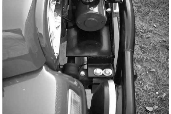
Above photo reflects winch plate mounting - Passenger side TJ*
