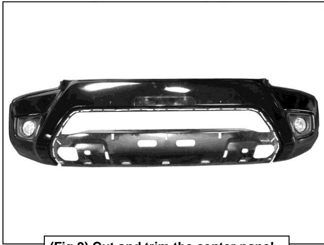
(Fig 9) Cut and trim the center panel to allow installation of Hiline Bumper
