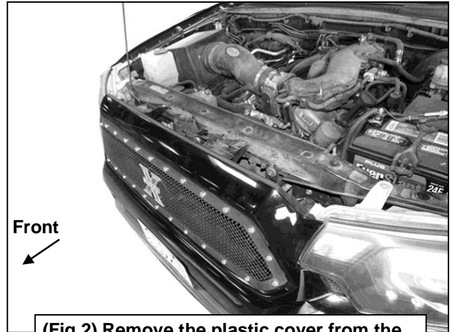
(Fig 2) Remove the plastic cover from the top of the radiator. Remove grille assembly
